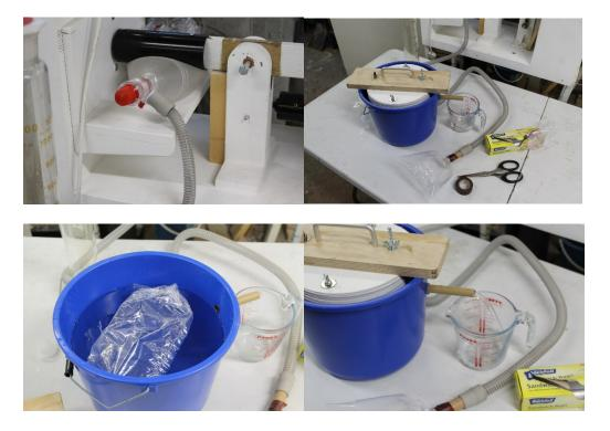
This method although simple in concept, is surprisingly consistent in providing a measured air volume scale for reference and allows for reasonably accurate calibration for inconsistencies both in build accuracy, and in the make of BVM to be utilised.
